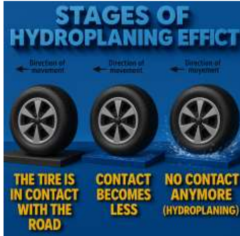
Figure 2. Stages of aquaplaning
