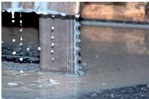
Fig. 4. Band bimetal saws for metal made of high-speed steel M51
