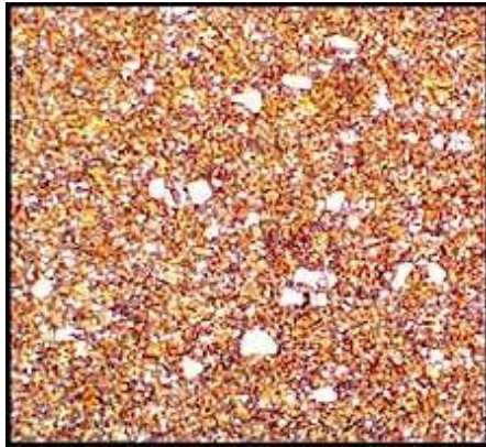
Fig. 2. Microstructure of M51 steel (12P10M4K10)
